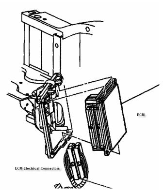
Fast Idle provides an elevated engine speed control to one setting. It is not to be used if any hydraulic application is intended. Fast Idle requires hard-wiring into the Powertrain Control Module (PCM) and the use of a momentary type switch. The ECM is easy to access and does not require removal of the TCM. A 7mm bolt retains each of the two connectors to the ECM.
