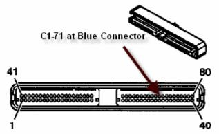
2. You'll need to gently squeeze the retainers holding the clear 'blue' sleeve from the C1 white insert so you can slide the terminal and wire to location 71 on C1 from the harness side of the C1 connector. Re-install the blue sleeve making sure that your added pin has retained its new location. Reconnect your blue connector C1 to the ECM when you've finished.
