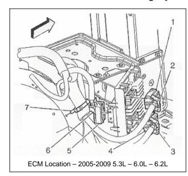
Disengage the engine wiring harness upper electrical connector retainer (2) and remove the connector (1) from the ECM.
