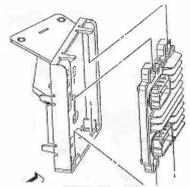
Disengage the retainer tabs securing the ECM to the bracket. Remove the ECM.
