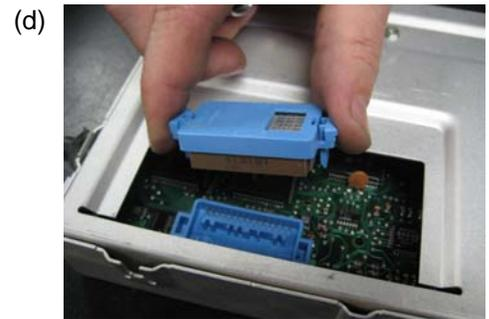
5. The Westers MEMCAL should look like (e). Press the Westers MEMCAL into the computer as in (f). There is no way to install this backwards so if it doesn't go in, turn it around.
