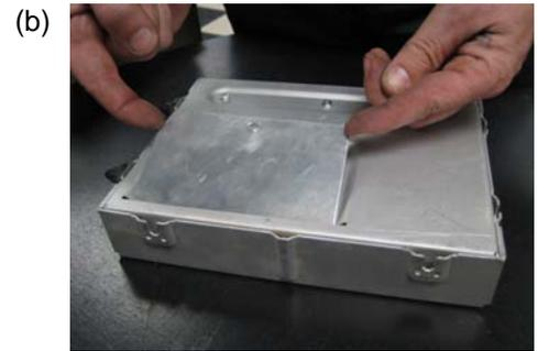
4. Place fingers on each side of the MEMCAL (c), squeeze clips together to release the MEMCAL (d).
