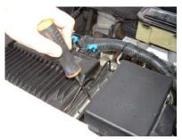
Step Three: Use a screwdriver (or tool of your preference) to aid in the release of your computer from its mounting bracket.
