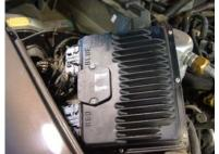
Step Eight: Flip the computer over so that the underside is up.
