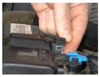
Step Six: Depress the release tab of the connector to remove all electrical connections.
