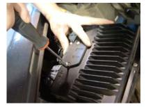
Step Nine: Use a torx screwdriver to remove the small panel on the back of the ECM.
