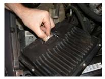
Step Eleven: Squeeze the white release tabs as shown to remove the knock module.
